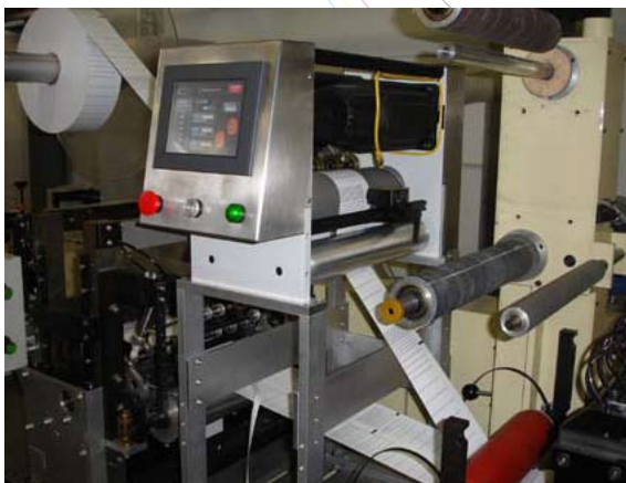
The Servo3000 can register a 2nd pre-printed web to the web already running in the press. Featured on a Gallus EM 340.
