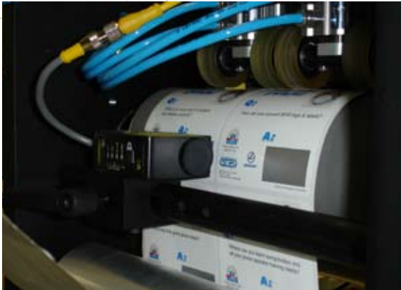
A close up view of the coated pacing roll and gripper wheels to prevent web slippage. Also shown is the print mark sensor.
