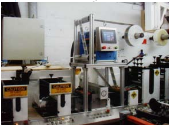
Laminating a pre-printed web is a simple way to produce coupons, booklets, and game pieces. Featured on an Aquaflex InstaPrep.
